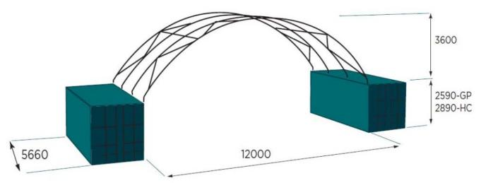
Base Rails included as a standard design feature on every Container Dome
